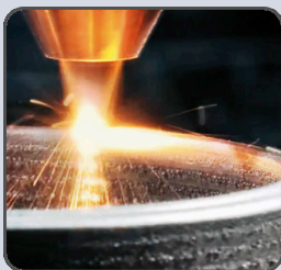
Additive manufacturing monitoring
