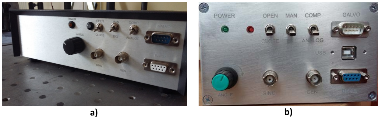
Fig.3 Front panel of shutter controllers, a) old version, b) new version with additional option for operation in “Master” mode (“SINC” output) and USB port.
